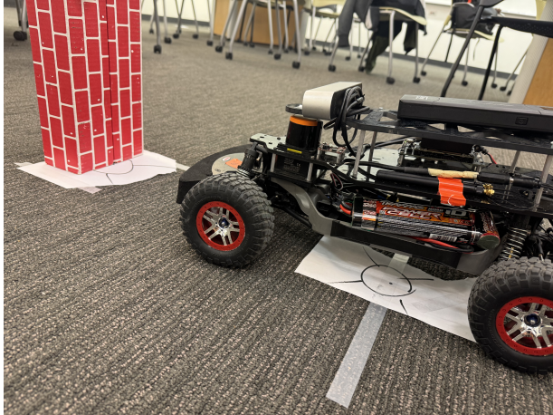
Figure 13: We measured the distance from the center of the LiDAR to the point on the ground to see how far it overshoot.
