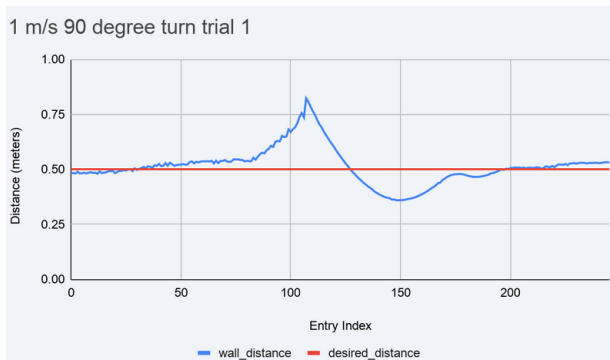
Figure 7: Plot of desired distance (red) and perceived distance (blue) as the robot makes an inward 90 degrees turn at 1 m/s
